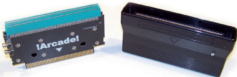
» MVS to AES converters (two different models pictured) allow AES owners to play relatively cheap MVS games on their AES consoles in lieu of forking over hundreds of dollars for rare AES originals.
